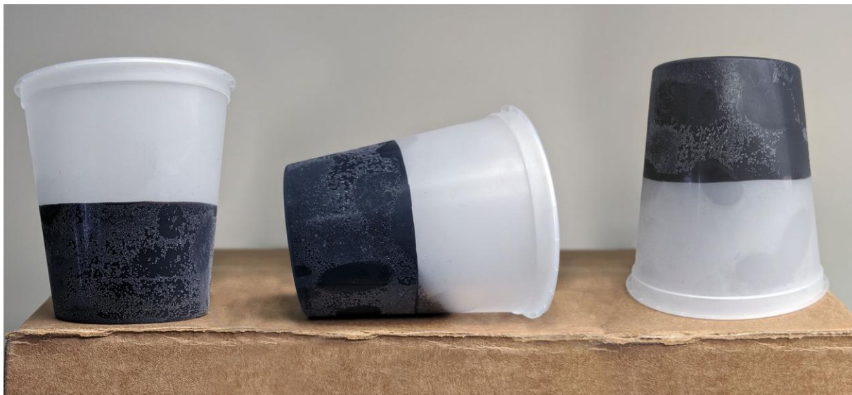
Figure 9: Crude oil viscosity increase demonstration at -25 °C.
