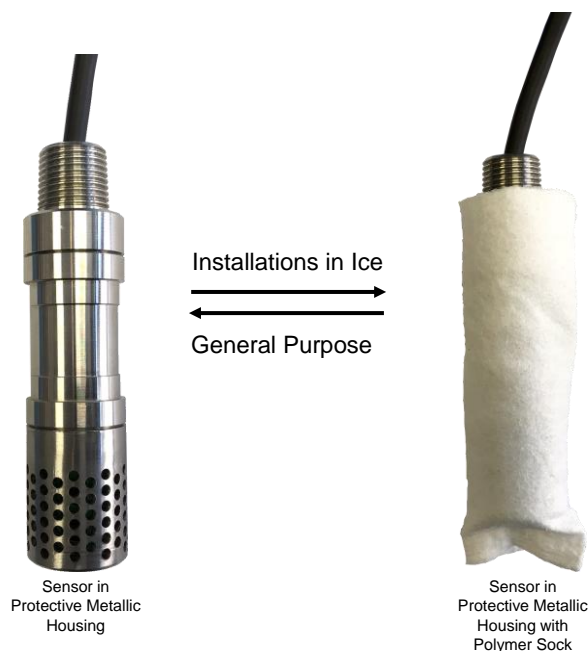
Figure 7: PA sensors in metal housing and polymer sleeve
